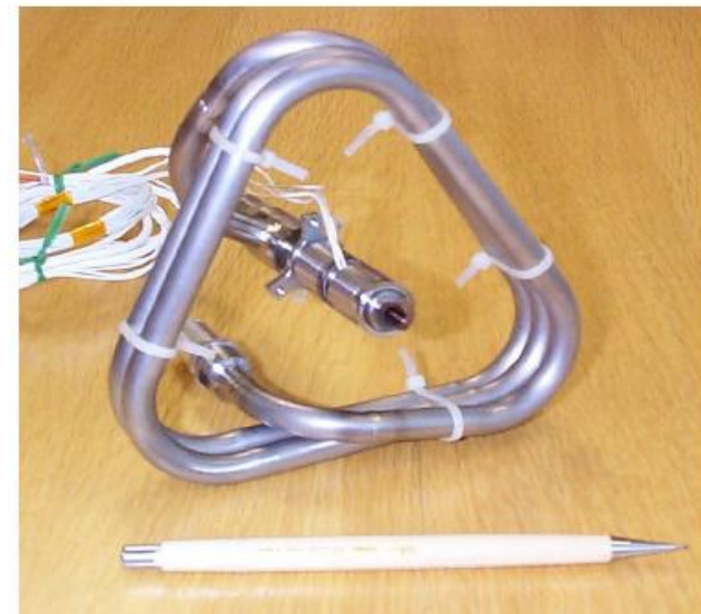
SNAP's Butane Propellant Orbit Control System Thruster
